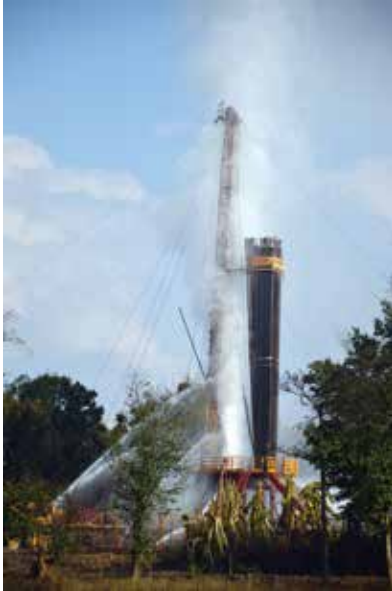
Well started releasing natural gas in an uncontrolled manner on 27th May 2020
