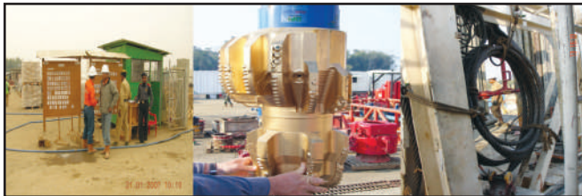
T CARD SYSTEM AT THE GATE BICENTER BIT AT WELL SITE COILING OF BULL LINE ON DERRICK FLOOR
